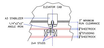
NOTE: STABILIZER IS MOST COMMONLY PLACED IN MIDDLE OF WALL OPPOSITE THE RAIL. IF THERE IS AN OPENING ON THAT WALL THE STABILIZER MAY BE RELOCATED TO WALL ADJACENT TO THE RAIL.
