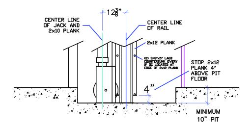
6" MINIMUM 3000 PSI REINFORCED CONCRETE #4 AT 12" O.C. EACH WAY.
